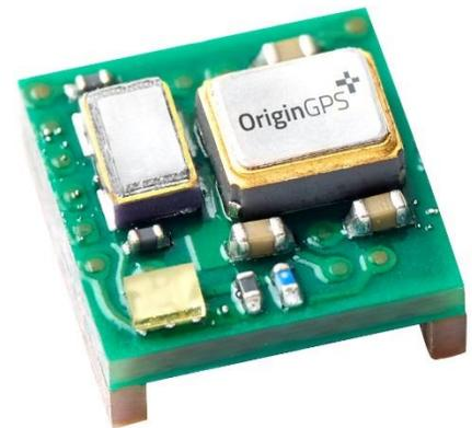
Utilizing MediaTek's MT3333 chip, the Multi Micro Hornet extends the functionality of GPS and GNSS solutions in wearables, drones and Internet of Things devices, providing a highly integrated multi-GNSS solution that delivers the world's smallest footprint, without sacrificing any of its superior power consumption, signal sensitivity and accuracy.
