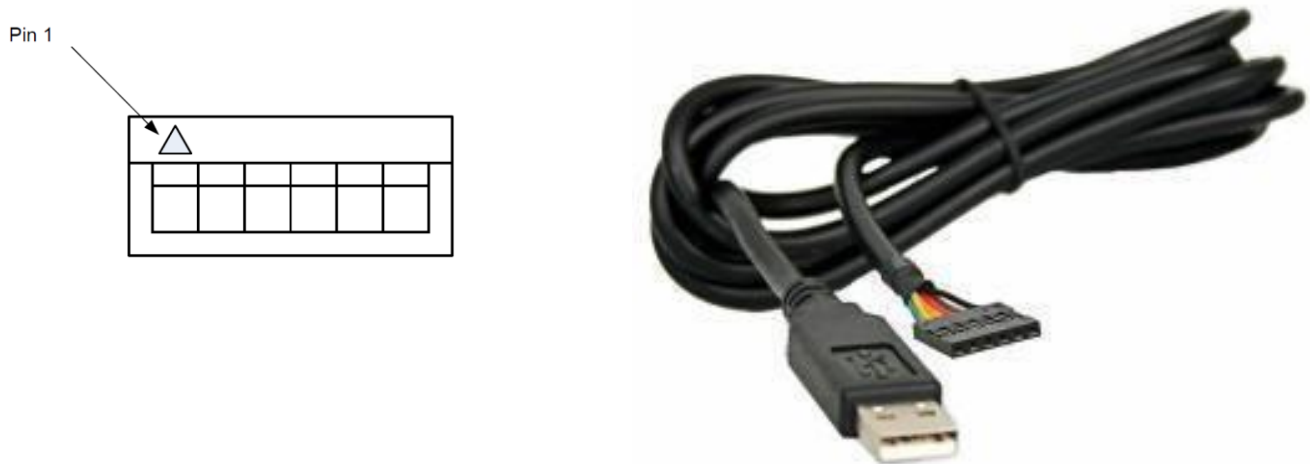
FIGURE 13 - PIN HEADER SOCKET BOTTOM VIEW
